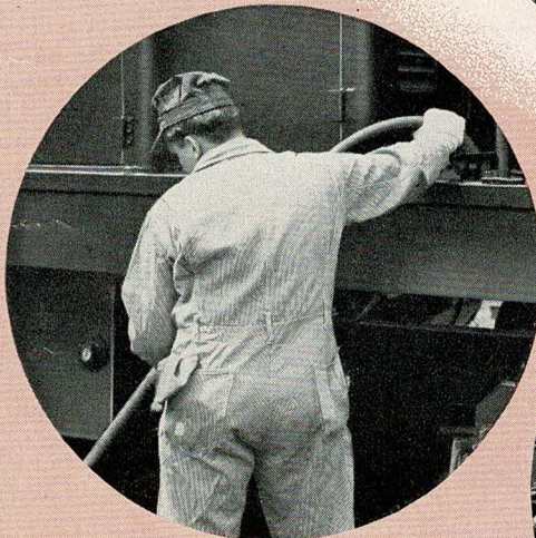
Fuel-filling pipes and level gages are conveniently located for fast refueling from the ground.
