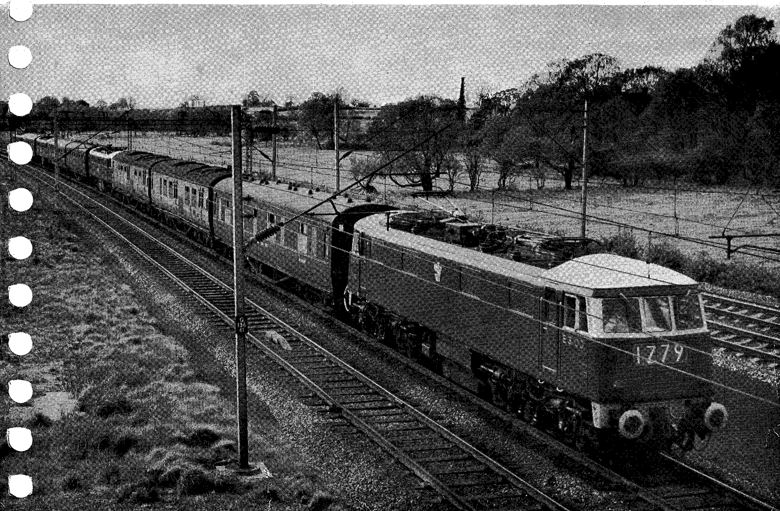
Fig 1 An 'English Electric' 25kV ac locomotive hauling a dynamometer car and test units between Crewe and Stafford, May 1963. The three other electric locomotives included in the train are rheostatically braked
