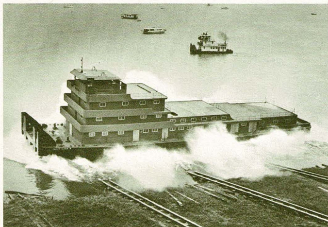
Launching of the Patrick Calhoun, Jr., a modern Mississippi River towboat that is powered by four Alco 12-cylinder Model 251 diesel engines.
