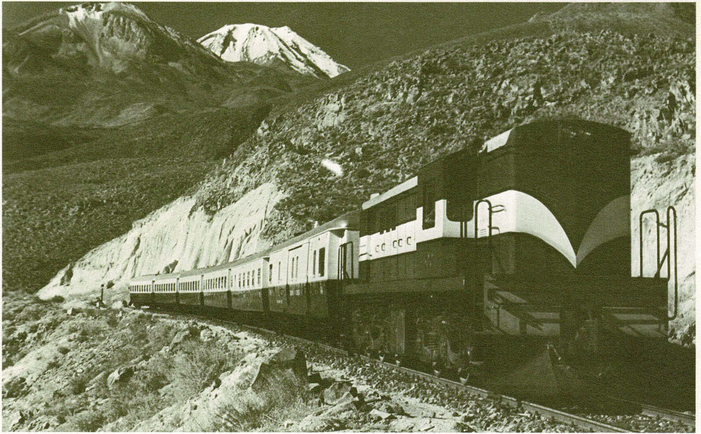
Alco DL-531 unit hauling a passenger express across the Peruvian Andes at 14,688 feet above sea level. Other Alco units operate efficiently in Peru at altitudes in excess of 16,500 feet.
