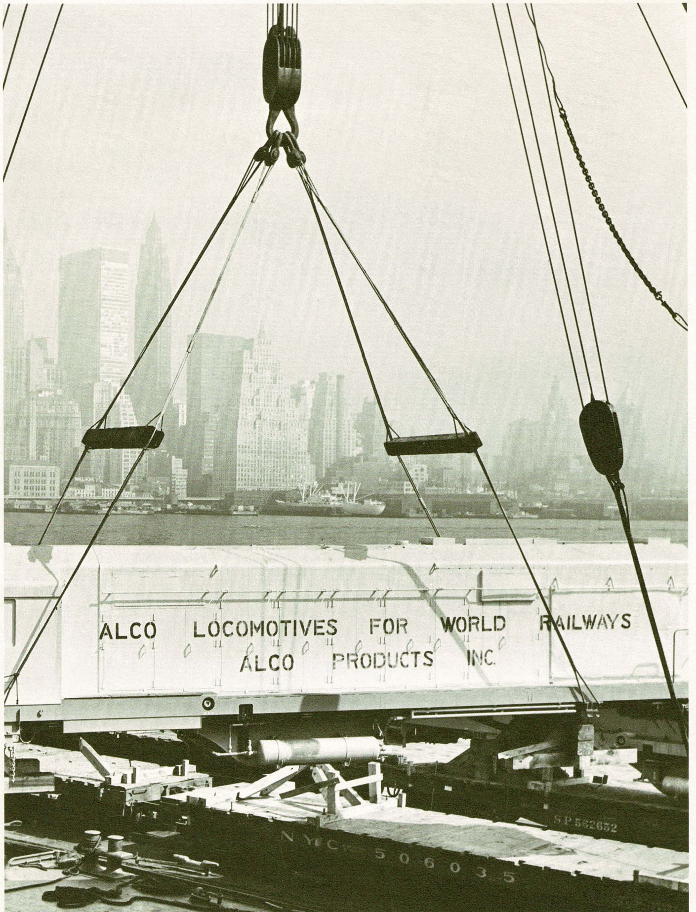
An Alco DL-560 locomotive, wrapped in a protective cocoon, is hoisted from a Port of New York pier. Destination: India.
