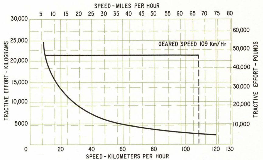
Tractive Effort Characteristics with 914 mm (36") Wheels and Basic 92:19 Gearing.
